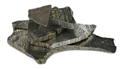
Similar to iron, cobalt too can be magnetized, resulting in the production of some incredibly strong magnets such as samarium-cobalt (SmCo) magnets, which are extremely resistant to demagnetization. Cobalt and its alloys are also used in hard disk drives and MRI machines as well as in the dry batteries of modern cars. The scarcity of cobalt can cause the price of this element to fluctuate, making it a less desirable choice for some industries.
