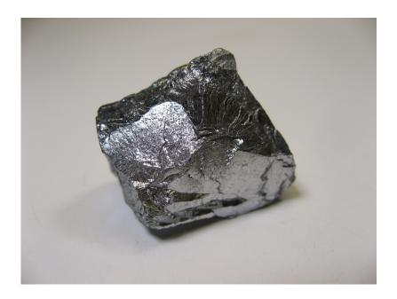
Chromium resists corrosion because of an oxide layer that forms on its surface when it comes into contact with oxygen in the air. Chromium's incredibly shiny and aesthetically pleasing finish is due to the fact that the metallic structure of chromium metal is incredibly uniform and absorbs and reemits light without being scattered.
