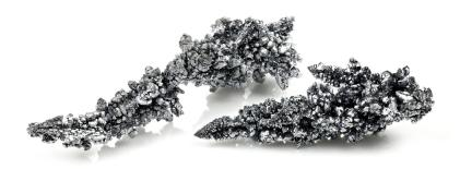
Vanadium is used as an additive metal in some types of steel. Steels that contain metals such as vanadium and chromium are more hardenable.
