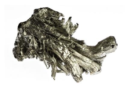
We can make metals stronger by mixing them with other metals to create alloys. Small amounts of scandium ( $\sim$  2%) can be mixed with large amounts of aluminum to make an alloy that has high mechanical strength, high ductility, and improved corrosion resistance. These metal alloys are light and very hard.
