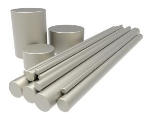
One of the primary uses of titanium is in the production of titanium-aluminum alloys. These alloys are used heavily in the production of aircraft, armor plating, and even spacecraft! When titanium is alloyed with aluminum, vanadium, and other elements, the alloys produced have high tensile strength but are also relatively lightweight and can withstand high temperatures without being damaged.
