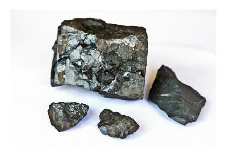
Perhaps manganese's most important use is in the production of steel where it is considered to be of critical importance, as there is no satisfactory substitute for manganese in many applications of metallurgy. When alloyed with iron, ferromanganese is formed. Ferromanganese is used as an additive in many different types of steel. On its own, manganese is a very brittle material, so it is more useful as an alloy.
