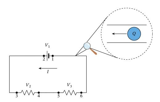
We can calculate the work done on the positive charge as it moves between points 1 to 6 of the circuit. The work done is equal to the magnitude of the charge multiplied by the potential difference across the points it travels between. This is equal to the change in the electrical potential energy of the charge and can be visualized on the following graph of electrical potential energy, E, against distance traveled around the circuit, d.
