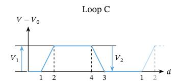
As before, across a whole loop, the work done on the charge, and therefore the total potential difference across each component in the loop, must equal zero. This means that Kirchhoff's second law can be applied to any loop in a circuit.
