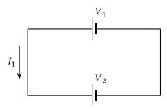
If the magnitude of  $V_1$  is not equal to that of  $V_2$ , then the loop appears to not follow Kirchhoff's second law; this is not possible, as energy must always be conserved! In that case, there is an internal resistance in each battery that must be considered that causes the drop in potential required to conserve energy in the circuit.
