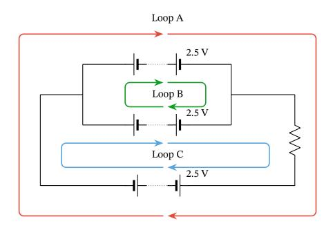
To find the decrease in potential across the resistor,  $V_R$ , we can look at either loop A or loop C.
