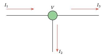
The amount of energy into the node per unit of time, the power in, is equal to the sum of currents into the node multiplied by the voltage of the node, V:
