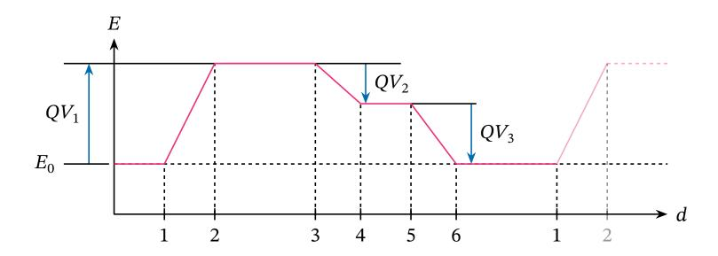
Note that the work done on the charge only tells us the *change* in electrical potential energy; the charge has some base level of electrical potential energy of  $E_0$ .
