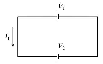
If the magnitude of  $V_1$  is not equal to that of  $V_2$ , then the loop appears to not follow Kirchhoff's second law; this is not possible, as energy must always be conserved! In that case, there is an internal resistance in each battery that must be considered that causes the drop in potential required to conserve energy in the circuit.
