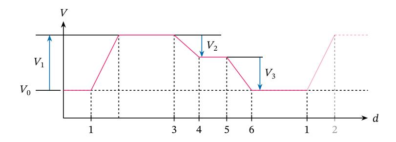
Note that there is some base-level electrical potential of the charge,  $V_0$ ; we can only measure potential difference between two points in the circuit.
