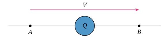
The charge moves because the potential difference causes a force to act on the charge, which does work on it as it moves. The work done on the charge, E, is equal to the charge multiplied by the potential difference between the two points:
