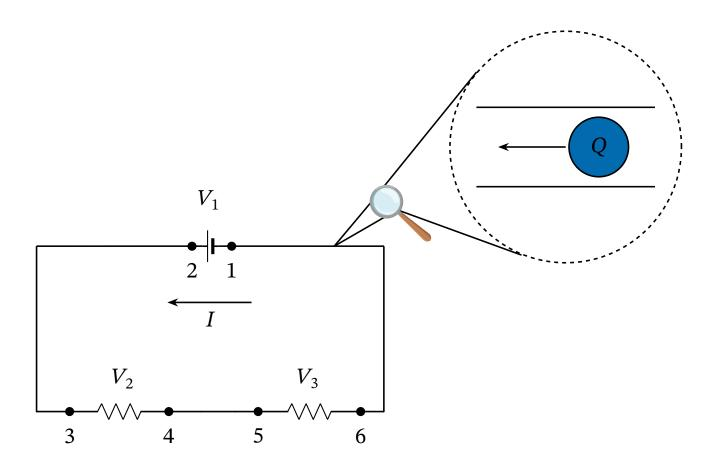
We can calculate the work done on the positive charge as it moves between points 1 to 6 of the circuit. The work done is equal to the magnitude of the charge multiplied by the potential difference across the points it travels between. This is equal to the change in the electrical potential energy of the charge and can be visualized on the following graph of electrical potential energy, E, against distance traveled around the circuit, d.
