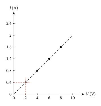
Using the equation  $R = \frac{V}{I}$  and substituting 2 V for V and 0.4 A for I, we find
