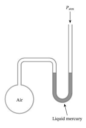
Air will fill the spherical container if it is not filled with some other type of liquid. The air will exert pressure on the mercury from one side while the atmosphere exerts pressure from the other side. The right- and left-hand side mercury levels will be elevated to the same height because the pressure from the atmosphere is equal to the pressure from the air inside the spherical container.
